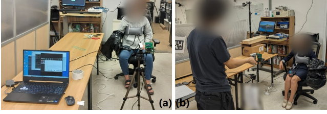
Figure 4: Experiment scenarios: (a) tripod, (b) handheld. operate at 50Hz, producing D_{heart} \in \mathbb{R}^{1 \times 50t} and D_{breath} \in \mathbb{R}^{1 \times 50t} . These sensors connect to a NeuLog USB streaming unit, controlled via an HTTP API on a Windows laptop.
